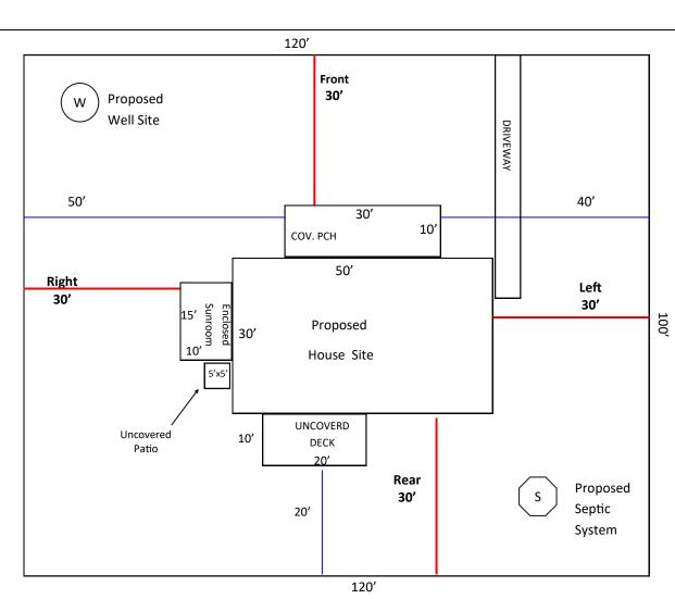
**\*\* Note:** The site plan does not have to be to scale and can be hand drawn, but must show the configuration of the proposed lot.
